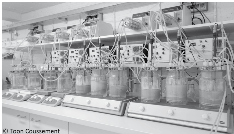
Fig. 2 Simulator of the Human Intestinal Microbial Ecosystem (SHIME)
