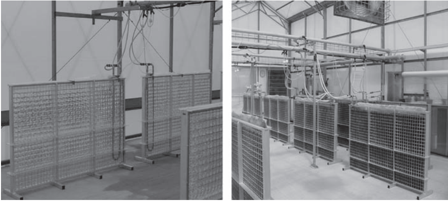
Fig. 2 On the left, the DFPP design showing different elements; on the right, green stage of Haematococcus cultivated in the DFPP
